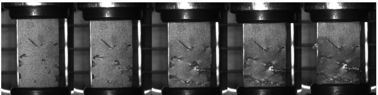
Fig 1: Sequence of loading phases, showing the concrete specimen under increasing compression.
