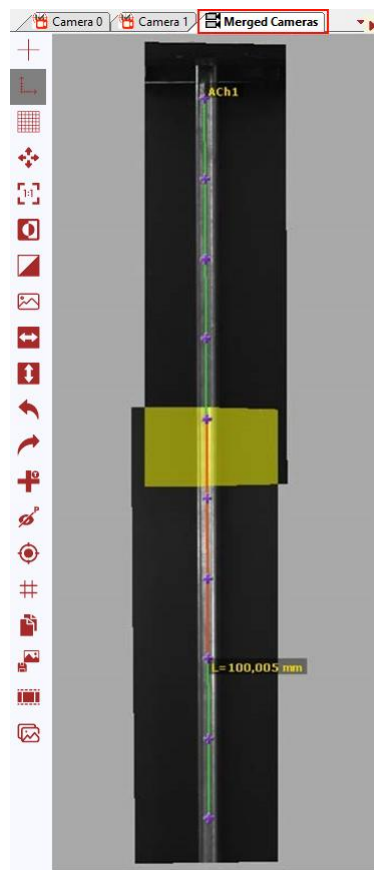
Figure 48: Stitched mono mode – two cameras for FOV extension (an overlap between cameras is coloured yellow) scene
