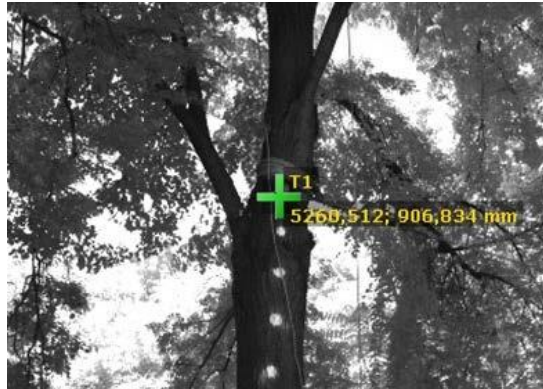
Figure 52: A point probe (the measurement of the bending displacement of a tree)
