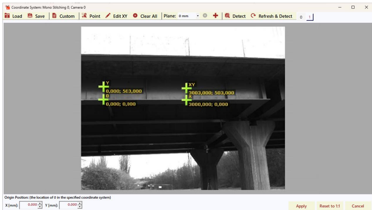
Figure 49: Large object calibration in a stitched mono scene
