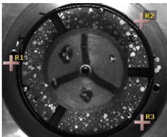
Figure 54: Rigid plane probes (applied on the stator of a bearing)
