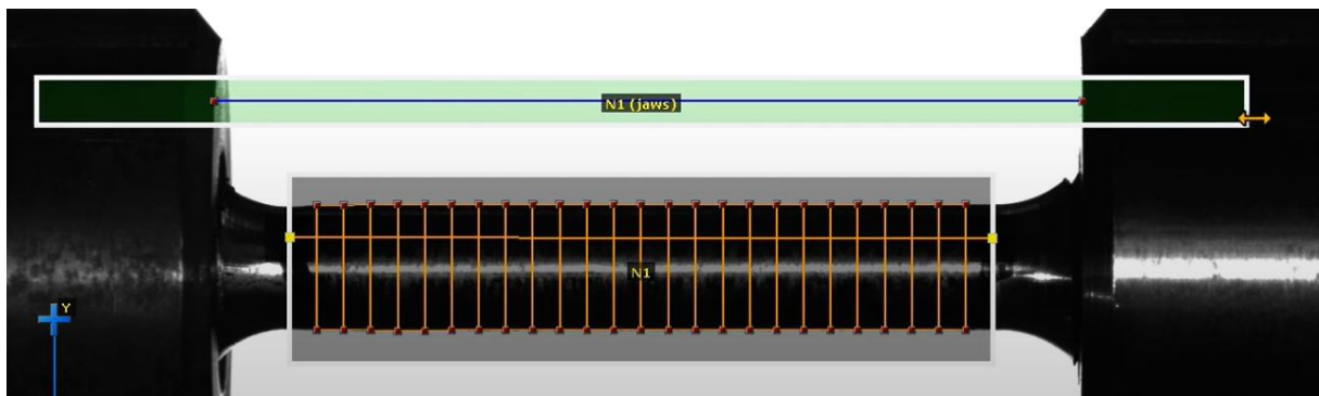
Figure 62: Neck gauge – detect jaws feature
