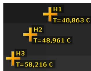
Figure 53: A thermal probe used for temperature readout at specific locations in the image
